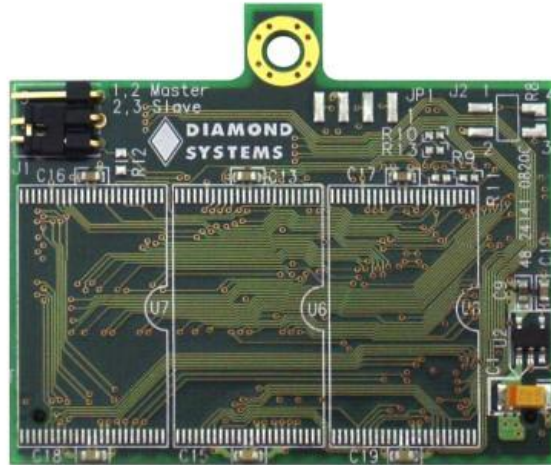
IDE Flashdisk (top side view; IDE connector is underneath)
